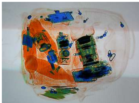
FIGURE 30.24 This x-ray image shows the contents of a piece of luggage. The denser the material, the darker the shadow. (credit: IDuke, Wikimedia Commons)
