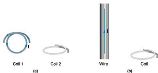
FIGURE 23.53 (a) The planes of the two coils are perpendicular. (b) The wire is perpendicular to the plane of the coil.
