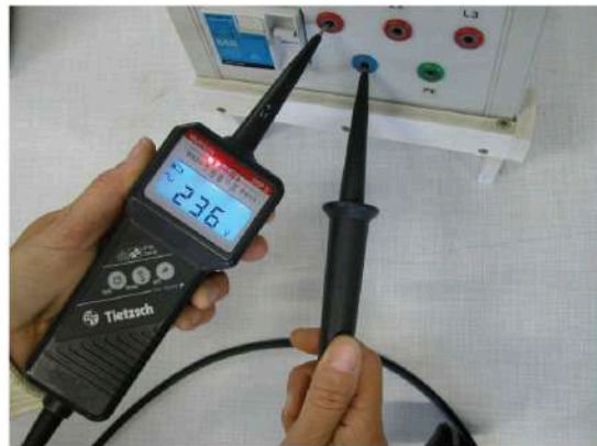
FIGURE 21.27 (a) To measure potential differences in this series circuit, the voltmeter (V) is placed in parallel with the voltage source or either of the resistors. Note that terminal voltage is measured between points a and b. It is not possible to connect the voltmeter directly across the emf without including its internal resistance, r . (b) A digital voltmeter in use. (credit: Messtechniker, Wikimedia Commons)
