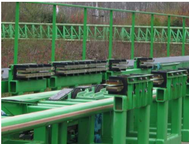
FIGURE 23.18 The rows of rare earth magnets (protruding horizontally) are used for magnetic braking in roller coasters. (credit: Stefan Scheer, Wikimedia Commons)
