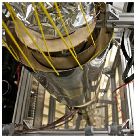
FIGURE 1.17 An atomic clock such as this one uses the vibrations of cesium atoms to keep time to a precision of better than a microsecond per year. The fundamental unit of time, the second, is based on such clocks. This image is looking down from the top of an atomic fountain nearly 30 feet tall! (credit: Steve Jurvetson/Flickr)
