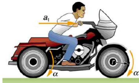
FIGURE 10.6 The linear acceleration of a motorcycle is accompanied by an angular acceleration of its wheels.
