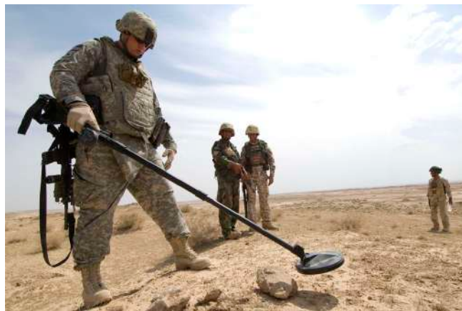
FIGURE 23.17 A soldier uses a metal detector to search for explosives and weapons. (credit: U.S. Army)
