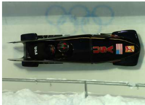
FIGURE 5.7 From racing cars to bobsled racers, aerodynamic shaping is crucial to achieving top speeds. Bobsleds are designed for speed. They are shaped like a bullet with tapered fins. (credit: U.S. Army, via Wikimedia Commons)
