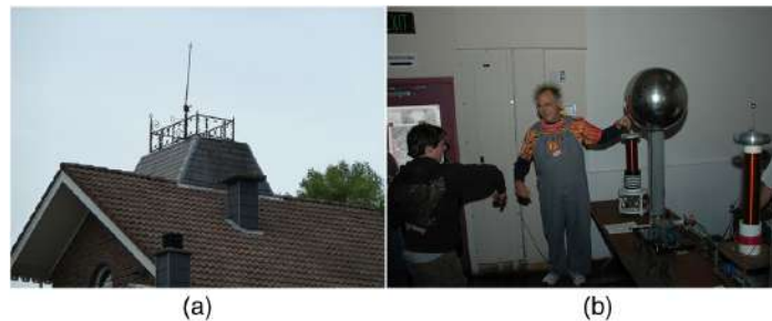
FIGURE 18.33 (a) A lightning rod is pointed to facilitate the transfer of charge. (credit: Romaine, Wikimedia Commons) (b) This Van de Graaff generator has a smooth surface with a large radius of curvature to prevent the transfer of charge and allow a large voltage to be generated. The mutual repulsion of like charges is evident in the person’s hair while touching the metal sphere. (credit: Jon ‘ShakataGaNai’ Davis/Wikimedia Commons).
