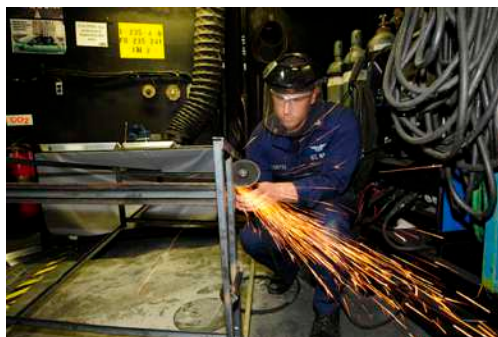
FIGURE 10.13 The motor works in spinning the grindstone, giving it rotational kinetic energy. That energy is then converted to heat, light, sound, and vibration. (credit: U.S. Navy photo by Mass Communication Specialist Seaman Zachary David Bell)
