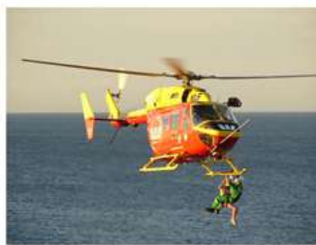
FIGURE 10.17 The first image shows how helicopters store large amounts of rotational kinetic energy in their blades. This energy must be put into the blades before takeoff and maintained until the end of the flight. The engines do not have enough power to simultaneously provide lift and put significant rotational energy into the blades. The second image shows a helicopter from the Auckland Westpac Rescue Helicopter Service. Over 50,000 lives have been saved since its operations beginning in 1973. Here, a water rescue operation is shown. (credit: 111 Emergency, Flickr)
