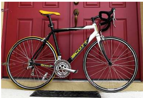
FIGURE 10.30 The image shows a side view of a racing bicycle. Can you see evidence in the design of the wheels on this racing bicycle that their moment of inertia has been purposely reduced? (credit: Jesús Rodríguez)
