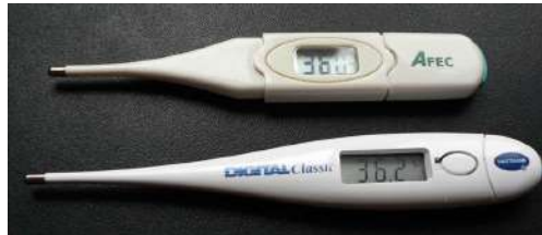
FIGURE 20.12 These familiar thermometers are based on the automated measurement of a thermistor's temperature-dependent resistance. (credit: Biol, Wikimedia Commons)
