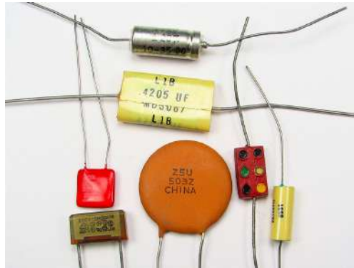
FIGURE 19.14 Some typical capacitors. Size and value of capacitance are not necessarily related. (credit: Windell Oskay)
