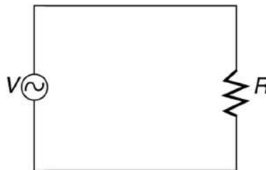
FIGURE 23.29 Schematic of a simple AC circuit with a voltage source and a single appliance represented by the resistance R . There are no safety features in this circuit.
