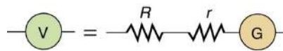
FIGURE 21.29 A large resistance R placed in series with a galvanometer G produces a voltmeter, the full-scale deflection of which depends on the choice of R . The larger the voltage to be measured, the larger R must be. (Note that r represents the internal resistance of the galvanometer.)
