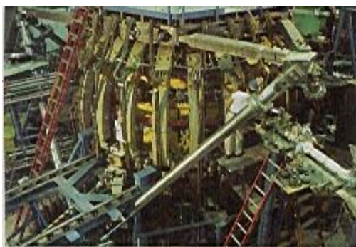
A tokamak apparatus, designed to generate the magnetic field necessary for containing a fusion reaction.
